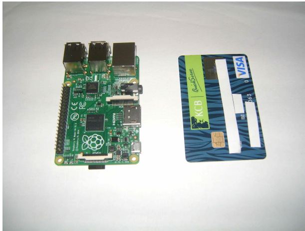
Figure 1: The Raspberry Pi. A Kenyan bank card is shown for comparison.
